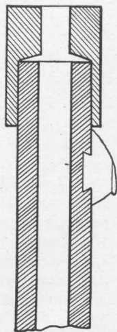
Figure 8. Design for muzzle guard
